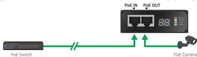
[The ITS-100 tester is connected at the end of the LAN cable, on the side of the PoE (PD) camera]
