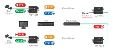
Transmission distance may vary depending on the type and quality of cable, use of power and environmental condition.
