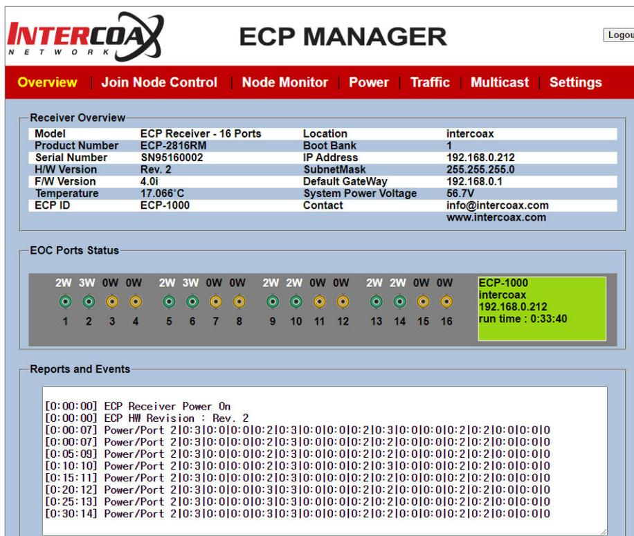
The dashboard for ECP Manager. It includes a navigation menu with options: Overview, Join Node Control, Node Monitor, Power, Traffic, Multicast, and Settings. The main content area is divided into three sections: Receiver Overview, EOC Ports Status, and Reports and Events.
